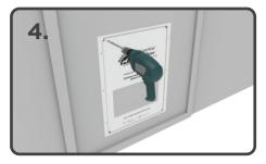
Drill a hole in each of the 4 inside corners with a minimum of 10mm (0.4") drill bit.
