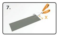
Measure thickness of door/panel and add 10mm (3/8") (x) so tunnel protrudes each side.
