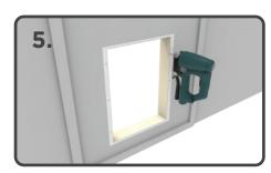
Using a reciprocating jigsaw, cut along marked lines.
