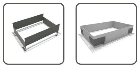
Fit all four partitions into outer door frame, use duct tape to secure the corners then place into opening.
