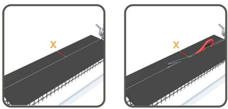
Measure the thickness of the door/panel and add 10mm (3/8") (x) so the tunnel protrudes 5mm (3/16") on each side. If required, cut partitions down to correct size.
