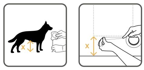
Measure the height (x) from the underside of the dog's stomach to the floor. Mark height (x) on door/panel with tape or similar. Adjust if necessary.
