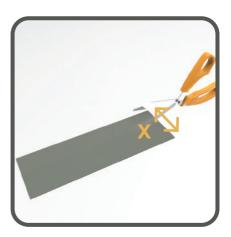
Measure the thickness of the door/panel and add 10mm (3/8") (x) so the tunnel protrudes 5mm (3/16") on each side. If required, cut partitions down to correct size.
