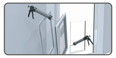
Refer to Steps 1 and 2 of "Installation". Place a bead of construction silicon around the internal section of the pet door and on the surface around the cut out to provide a weather seal. Tunnel partitions will need to be cut to size as per Step 6 of "Installation".
