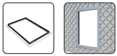
Fit all four partitions into outer door frame, use duct tape to secure the corners then place into opening. If the security screen has insect mesh, place a bead of construction silicon around the internal section of the pet door and on the mesh surface. Apply this around the cut out in order to hold the mesh in place when both frames are joined.
