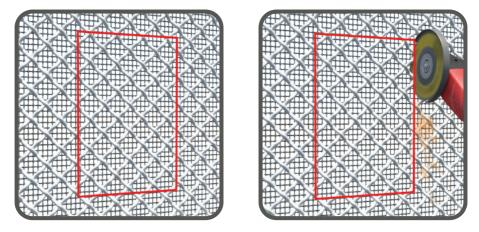
Take the measurements needed to cut the opening by following Steps 1-3 of the previous instructions. Using an angle grinder, cut out the opening.
