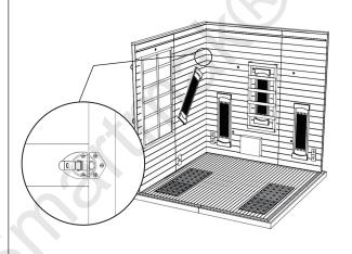
③ Place the other side panel and connect it to the back panel with buckles.
