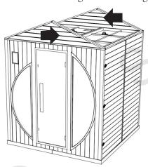
2 Install roof Place the two roof pieces one behind the other.
