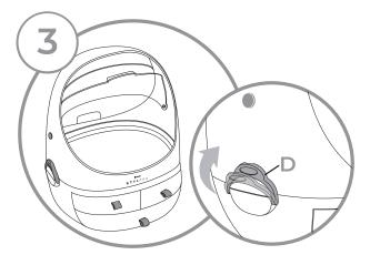
Secure both sections by clipping each side of the pod together until the **Clips (D)** snap into position. These can separate as you wish.
