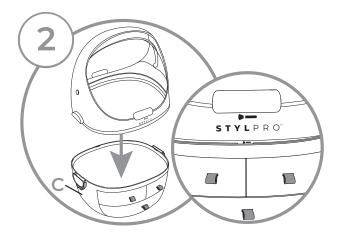
Parts **A** and **B** will now be held together and should not come apart. Place onto the lower **Base (C)** with the logos facing the same direction as the drawers.
