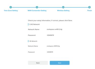
Note: After this setting, the router will reboot again. Go to your WI-FI network list and find the SSID named by yourself. The WiFi-enabled devices can connect to the AX1800 router by entering the new password. And the wired devices connected to the router can access the internet directly now. If you want to modify the settings, please log in the management page (IP address is 192.168.1.1) again after completing the initial settings.
