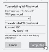
**Note:** By default, the extended network uses the same wireless network name (SSID) as your router. Change the extended SSID if you need.
