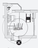
Too close to the router, extended Wi-Fi signal can not cover the dead zone.
