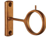
EB7 steel eyelet bracket, single 3 1/2" return, 1"W x 3 1/2"L backplate, eyelet 2 3/8"ID
