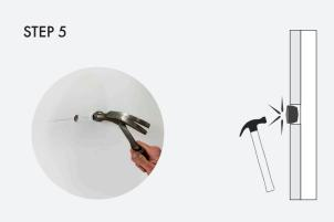
Insert the Gripit fixings into the holes. Use a hammer to gently tap them flush with your wall.
