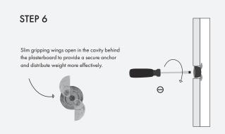
Use a flat head screwdriver to turn the cam and open the wings for super grip strength on every fixing.
