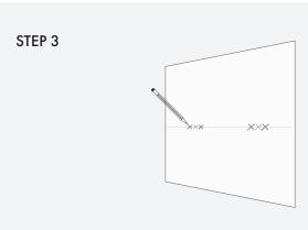
Hold the metal brackets against the markings on the wall and mark where the Gripit fixings need to go, making sure these are level all the way along.
