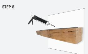
When you're happy with the positions of the beam, we recommend adding a small amount of silicone or grab adhesive to the back before re-installing. This is a precautionary measure and not absolutely necessary.
