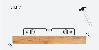
Place a spirit level on the mantel top to check it's level. Minor adjustments can be made by tapping the screws with a hammer.
