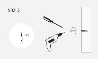
Use a PZ2 drill bit and drill or screwdriver to drive each screw into the wall plugs leaving them protruding approximately  $^{1}\!\!/_{2}$  of an inch.
