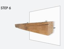
Place the beam onto the screws. The screws may need adjusting. When fitted correctly the beam will sit completely flush with the wall.
