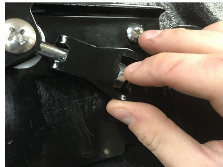
Turn square nut to adjust clamping pressure.
