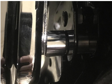
CORRECT mounting, brackets are butted up against chrome spacers and completely cover docking points
