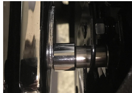
INCORRECT mounting, bracket is only halfway on to the docking points, not butted up to chrome spacer
