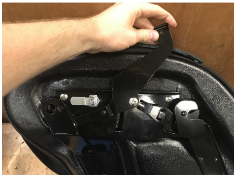
Move lever rearward (right in this picture) to make adjustments
