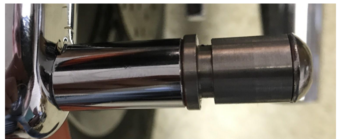
Correct stud mounting for rear strut holes
