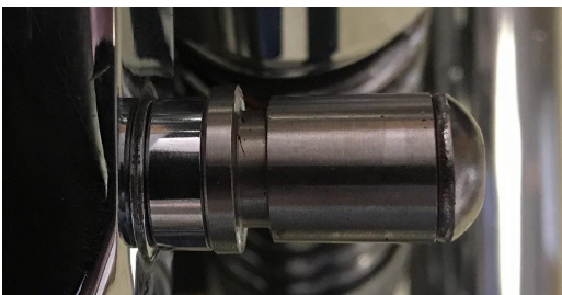
Correct stud mounting for front strut holes
