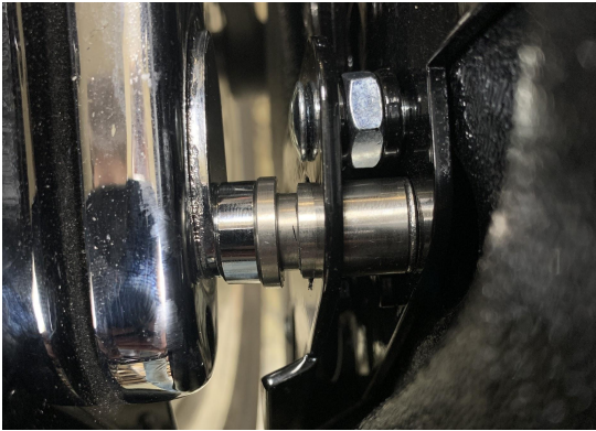
INCORRECT Brackets are not on the docking points and will not clamp on in this position
