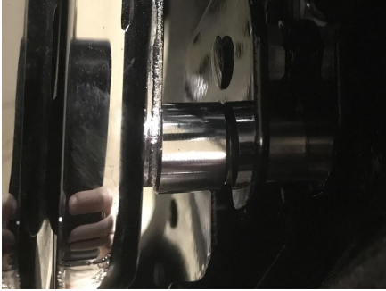
CORRECT mounting, brackets are butted up against chrome spacers (or Harley holdfast points) and completely cover docking points
