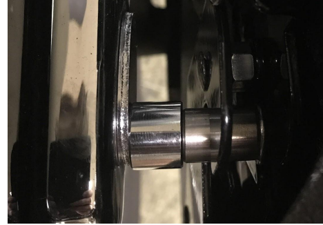
INCORRECT mounting, bracket is only halfway on to the docking points, not butted up to chrome spacer (or Harley holdfast points)
