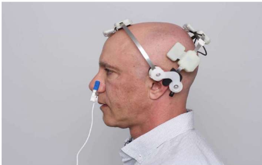
The device works using LEDs to shine near-infrared light directly into the brain. CREDIT: VIELIGHT
