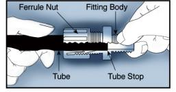
Refer to this diagram when inserting the tubing into the ferrule nuts
