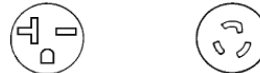
NEMA 6-20R (Straight) NEMA L6-20R (Locking) Outlet Configurations - 20 Ampere, 220 to 240 Volts Nominal
