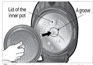
6 When putting the cover into the lid, press the cover handle after fitting the handle into the groove indicated by the arrow.
