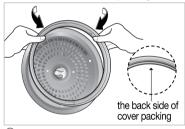
(5) When you fix the rubber packing into the detachable cover, hold it between and put it in the edge of the detachable cover by turning it.
