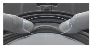
① As the Figure 1 shows, put the point #1 on the pressure packing with the standard notch #1 on the Inner Pot lid together before pressing the outer rim of the packing to insert it into the groove. Repeat with points #2 to #6.
