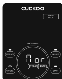
Before entering the temperature setting mode (when selecting the SLOW COOK menu)
