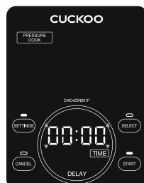
After entering the preset setting mode (when selecting the PRESSURE COOK menu)
