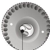
⑤ When you fix the rubber packing into the detachable cover, hold it between and put it in the edge of the detachable cover by turning it.
