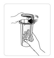
Match Safety switch unto the support groove and turn clockwise making sure it is tightly sealed.
