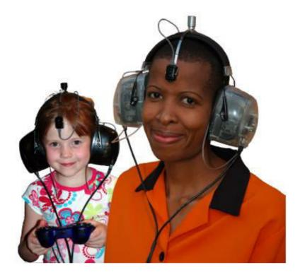
The ear-cups of this KUDUwave block out the ambient noise as a first attenuation barrier. At the bottom of each ear piece there are tubes at the end of which one can fit ear-tips. These tips are inserted into the ear of the patient and act as a second sound attenuation barrier. The ear-cups will then fit over these insert earphones through which sound is delivered to each ear of the patient.
