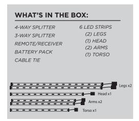
Take the battery pack and plug it into the remote receiver (don't turn on yet). Then plug the 4 way splitter into the remote receiver. Plug the 2 legs, torso and 3-way splitter into any of the 4 plugs. The 3-way splitter cable will be directly beneath the torso LED strip. The legs should face the opposite direction of the torso and 3-way splitter.
