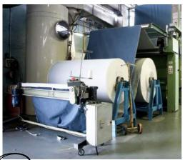
Dyeing) before dyeing starts, the dyeing recipe gets developed and approved via lab dips. On top of colours, you can adjust brushing and select add on finishing treatments. The list has 100+ options and some options are hard to figure out. These wet processes have some of the biggest environmental impact. So it is important to dye in Europe because regulation is much stricter.
