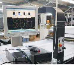
carment construction (typical "factory"): this is where your cutting patterns get developed, shrinkage for fabrics get calculated, the fabrics get cut, sent out to the print or embroidery house and then gets recollected to be assembled with sewing machines. For every different style of stitch, you'll need a different machine. The assembly line can reach up to 12 stations. These factories normally also do ironing, QC, and packing after all is completed.
