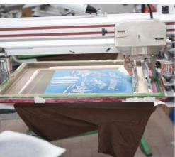
Printing these places hold large screen printing carousels with up to 16 colours or as a hybrid machines with digital printers included. If something with the screens is wrong and you print at a speed of 180 garments per hour, you're in trouble and you might suddenly have a massive delay affecting all following steps in the process.
