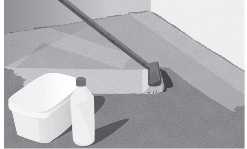
Fig.3. Clean and prime the floor
