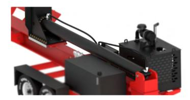
(5) PUSH BLOCK - The push block is what makes contact with the log when the 8" cylinder is in extension. ALWAYS ensure that your fingertips, hands, and/or loose clothing are a safe distance from the push block while it is in operation. NEVER alter/remove any nuts/bolts and/or fittings from the push block unless it is being serviced by a certified representative of Timberwolf Firewood Processing Equipment.
