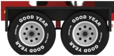
(9) FENDER - The TW-10 is equipped with two fenders. The TW-10's fenders protect the wheels and axles from unnecessary weathering and other damage.
