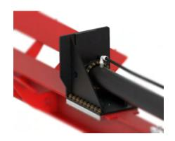
(6) TW-10 LEG - The TW-10 leg is constructed from 2.5" tubing and is secured by two 1" pins. This wide platform stabilizes the TW-10 while in operation. The TW-10 leg is NOT removable. If for any reason the 1" pins must be removed, ENSURE that they have been re-inserted prior to operation.
