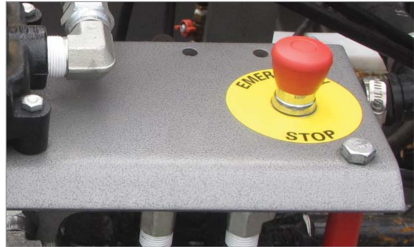
Emergency Shut Off Switch (“Panic Button”)
