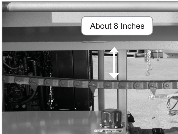
Feed Trough Chain Tension
