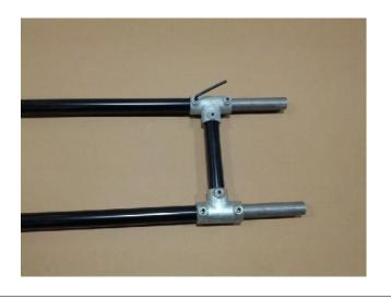
and into the pre-assembled center support, until they come to a stop against the ring-stoppers. Please note that the fit is intentionally very tight. You may have to slightly "wiggle" the horizontals to get them in place. LIGHTLY TIGHTEN set screws. Do NOT fully tighten the set screws at this point:
