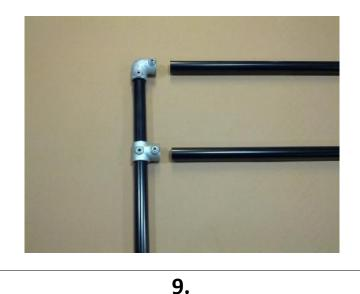
After visually ensuring they are square, fully tighten the preassembled barre end verticals on each side:
