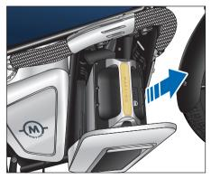
To install the primary battery, open the primary battery storage compartment, and carefully lift the battery and lower it into position.
