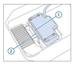
5. With the charging base unit aligned to the front retaining ledge, push the battery connector unit forward (1) and down (2) into the charging dock.
