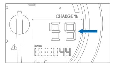
The battery's SoC can also be checked when the battery is not installed in the motorcycle by pressing the small button on the top of the battery. The SoC is displayed on the LED gauge, as shown below:
