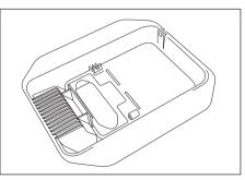
4. Align the long edge of the battery connector unit (1) with the front retaining ledge (2).
