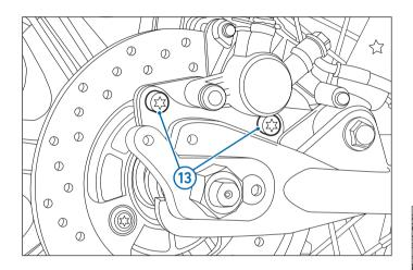
14. Secure the brake caliper to one side, using string or a retaining strap.
