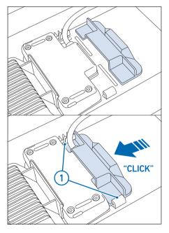
7. Once locked in position, you can remove the retaining lock by lifting the rear side of the lock upwards (1), which disengages the lock from the recess and sliding the lock away (2) from the battery connector unit.
