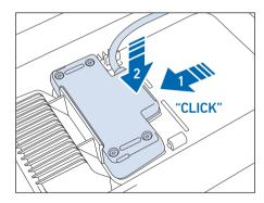
6. We are now going to fit the retaining lock. The retaining lock locates into two retaining brackets on the charging dock and locks the battery connector unit into position by clicking into a recess in the charging dock. Slide the retaining lock towards the battery connector unit, making sure the retaining lock locates under the retaining brackets (1) on the charging dock.
