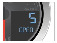
During the countdown period, press the battery storage compartment unlock button, located on the left-hand side handlebar switch, once (one long press) to unlock the battery storage compartment. Pull the handle outward to open the compartment.
