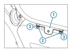
Align the pannier rail (1) to the upper and lower retaining brackets and loosely install the lower bolts (2) M6 x 12 mm (T30 Torx<sup>™</sup>) and the upper bolt (3) M6 x 10 mm (T30 Torx<sup>™</sup>).
