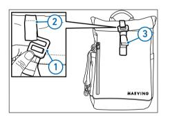
Press down on the locking clasp (1) on the pannier. Align the locking clasp (2) to the second bar and the retaining hook (3) to the third bar on the pannier rail (4).
