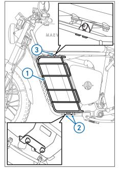
4. Tighten in the sequence shown to **8 Nm**.
