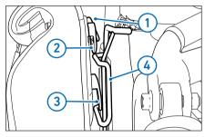
Lower the pannier to the pannier rail. Make sure the locking clasp (1) locks securely to the second bar (2) and the retaining hook (3) remains engaged with the third bar (4).
