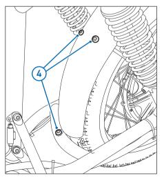
Remove the 2 bolts (T30 Torx<sup>™</sup>) and washers securing the rear mudguard supports to the swinging arm and detach the rear mudguard and light assembly.
