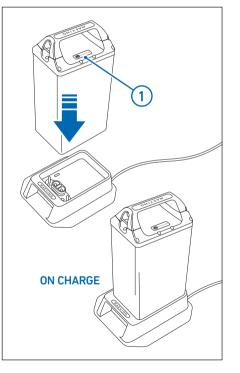
Leave the battery on the charging dock until it is either fully charged or has sufficient charge for your next journey. Once the battery is fully charged the battery charger will stop charging
