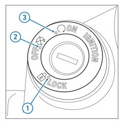
Always remove the ignition key when the motorcycle is parked, to reduce the chance of theft. The ignition key can be removed from the ignition barrel when the key is set to either **LOCK** or **OFF**.
