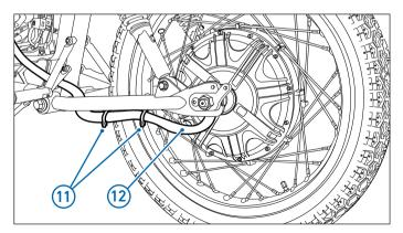
13. Remove the 2 bolts (T45 Torx<sup>™</sup>) securing the brake caliper and detach the rear brake caliper from the swinging arm.
