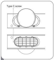
Insert the type C screw in the hole in the diffuser to prevent the diffuser from sliding out of the vent opening. If the diffuser is positioned correctly, the screw should just clear the edge of the opening in the vent panel. You should not have to drill through the vent panel.
