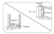
For window openings from 19" to 25", use the window vent panel (Panel A) and extension Panel B.
