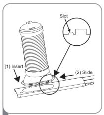
Align the tabs on the diffuser with the slots in the vent panel. Insert the diffuser into the opening in the vent panel and slide the diffuser all the way over to lock the tabs in place. Position the diffuser with the round opening above the bottom of the vent panel to avoid interference from the window sill.
