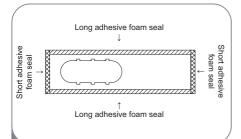
Attach the long adhesive foam weather seals to the top and bottom sides of the window vent panel assembly. Attach the short foam weather seals to the right and left sides of the panel assembly. (Attaching the foam weather seals to the panel assembly rather than the window sash and frame makes for easier cleanup when removing the panel assembly.)
