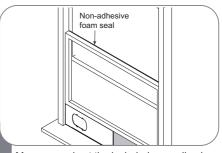
Measure and cut the included non-adhesive foam to fit the window opening. Stuff it between the window sashes to prevent air and insects from getting into the room.
