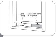
Insert the panel assembly in the bottom sash channel. Use care when installing the assembly, which will now fit very tightly in the opening. Close the sash tightly against the top of the panel assembly.
