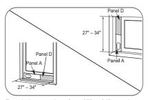
For window openings from 27" to 34", use the window vent panel (Panel A) and extension Panel D.
