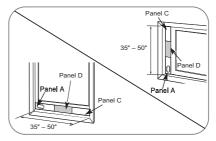
For window openings from 35" to 50", use the window vent panel (Panel A) and extension Panel C and Panel D.
