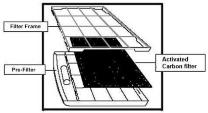
An optional  $3M^{TM}$  Antimicrobial Filter can also be purchased to replace the activated carbon filter. The  $3M^{TM}$  Antimicrobial Filter has an antimicrobial agent helps inhibit the growth of mold and mildew on the filter. This filter is electrostatically charged for enhanced particle capture and retention.
