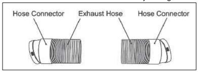
3. Align the slots on the hose connector to the tabs on the air intake / outlet and snap the hose to the unit.
