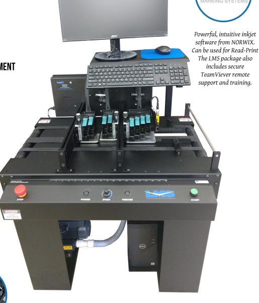
Split Head imagers with total: 4 Inches of print 2 inch on head 1 1+1 inch on head 2 for maximum flexibility
