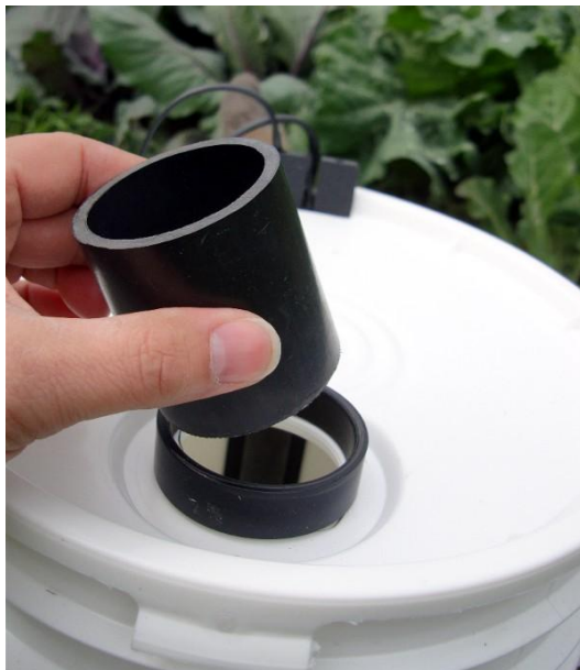
Bubble Breaker fits in the ring in the lid, with the screen facing down
