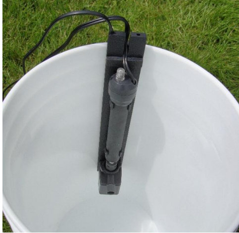
BioBlender hangs on the bucket rim
