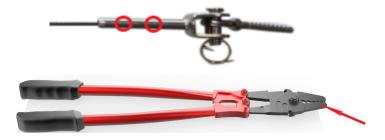
5. Measure the distance to the swage stud. Cut the cable accordingly. Insert the cable into the stud and swage twice using the cable crimper (die #2, then die #1). For long distances, swage three times.
