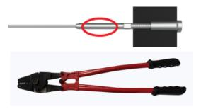
4. Measure the distance to the second swage stud terminal. Cut the cable accordingly. Insert the cable into the swage stud and swage twice using the cable crimper (die #1). For long distance, swage three times.
