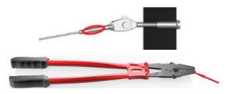
5. Measure the distance to the swage stud. Cut the cable accordingly. Insert the cable into the stud and swage twice using the cable crimper (die #2, then die #1). For long distances, swage three times.
