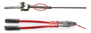
4. Measure the distance to the second swage fork terminal. Cut the cable accordingly. Insert the cable into the swage fork terminal and swage twice using the cable crimper (die #2, then die #1). For long distances, swage three times.
