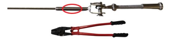
4. Measure the distance to the second swage fork terminal. Cut the cable accordingly. Insert the cable into the swage fork terminal and swage twice using the cable crimper (die #2, then die #1). For long distances, swage three times.
