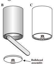
B) Spread a layer of epoxy around the inside circumference of the coupler to a depth of about 1/2".C) Push the bulkhead assembly into the coupler until it is about 1/4" past
