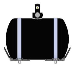
When installing the bottle into the car, it is advised that the bottle is mounted to anti vibration rubber mounts.
