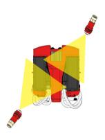
The nozzle positions play a key part in successfully bringing a fire under control & extinguishing it.
