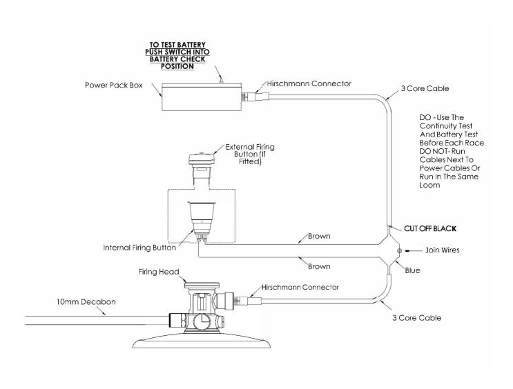
The wiring loom is 3 cable please note only the Blue and Brown are used, cut Black off.
