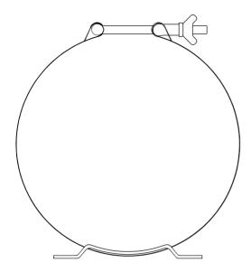
SP148 - 5" Cylinder Retaining Bracket
