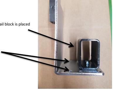
6. Bolts are placed at the bottom of the rail bracket going up. (Do not over tighten)
