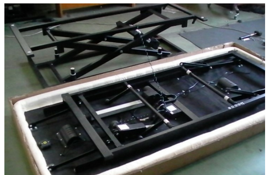
Electronic connection lifting motor completed.
