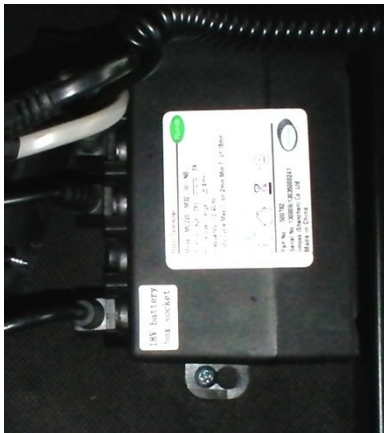
Empty socket on control box for connection of the Kalmia Perfect Height Bed system lifting motor.
