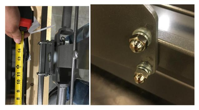
3. Tighten the nuts using a 9/16" wrench. Tighten evenly to secure the rail straight on the head section.
