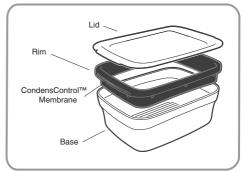
WARNING: Please do not remove, damage, or perforate the CondensControl™ membrane in the rim/lid as this will affect performance.
