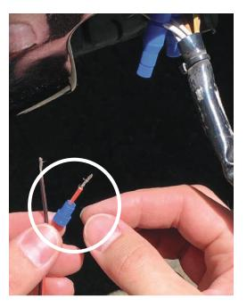
Unscrew the small end of the Posi-Tap connectors you installed in the previous step(s). Slide this over the wire as shown. Be sure to strip the lead wires for the next step.
