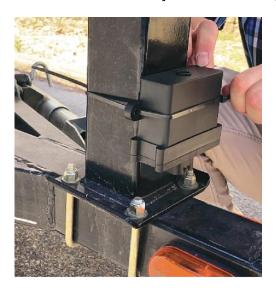
Using the provided double-sided tape AND cable ties, secure the TPMS Booster to your trailer.
