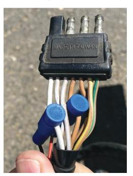
Connect the large end of the provided Posi-Tap connectors to the power and ground wires you have identified. Do this by unscrewing the large end of the Posi-Tap and then sliding it over the wire. Slide the tapping connector up onto the guide and tighten it down to pierce the wire.
