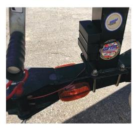
Route the harness to the power and ground source you identified and cut to length. Secure the harness with the provided zip ties.
