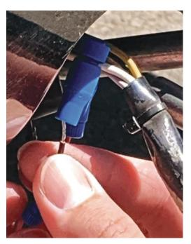
Slide the exposed end of each wire into the binding post area of the appropriate Posi-Tap.
