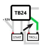
10. The GREEN cable connects to the negative (-) terminal of the Trolling battery. Extending this wire with 8- or 6-gauge wire can be done, if necessary.
