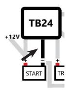
8. Connect the BLACK Trollbridge 24 ground (-) wire to the negative terminal of the starting battery. This terminal also connects to the negative (-) of the starting battery and the negative (-) side of the trolling motor. Extending this wire with 8- or 6-gauge wire can be done, if necessary.
