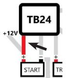
9. The RED cable is connected to the positive (+) terminal of Starting battery on a 2 battery system. On 3 battery systems this should be made to the positive (+) terminal of the House battery. Extending this wire with 8- or 6-gauge wire can be done, if necessary.
