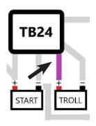
11. Connect the PURPLE (or WHITE) cable to the trolling motor battery positive (+) terminal. Extending this wire with 8- or 6-gauge wire can be done, if necessary.
