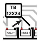
9. Connect the negative (-) terminal of the Trolling Battery 1 to the negative (-) terminal of the Starting battery. This terminal also connects to the ground wire of the engine and the negative (-) side of the trolling motor. Extending this wire with 8- or 6-gauge wire can be done, if necessary.
