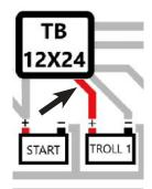
10. Connect the RED cable to the Trolling Battery 1 positive (+) terminal. **Shortening this cable will VOID the warranty.** Extending this wire with 8- or 6-gauge wire can be done, if necessary.
