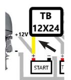
13. The YELLOW cable is connected to the positive (+) terminal of Starting battery.Shortening this cable will VOID the warranty. Extending this wire with 8- or 6-gauge wire can be done, if necessary.
