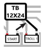
8. Connect the BLACK Trollbridge 12x24 ground (-) wire to the negative (-) terminal of the Starting battery. This terminal also connects to the ground wire of the engine and the negative (-) side of the trolling motor. Extending this wire with 8- or 6-gauge wire can be done, if necessary.
