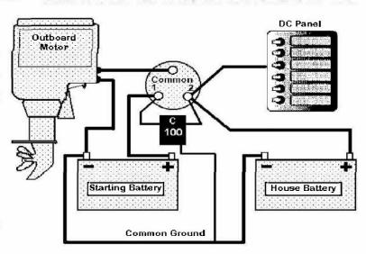
**WARNING:** If you use this circuit, turning the switch to "OFF" while the engine is running may damage your alternator. If not using a switch, the motor connects directly to the starting battery.
