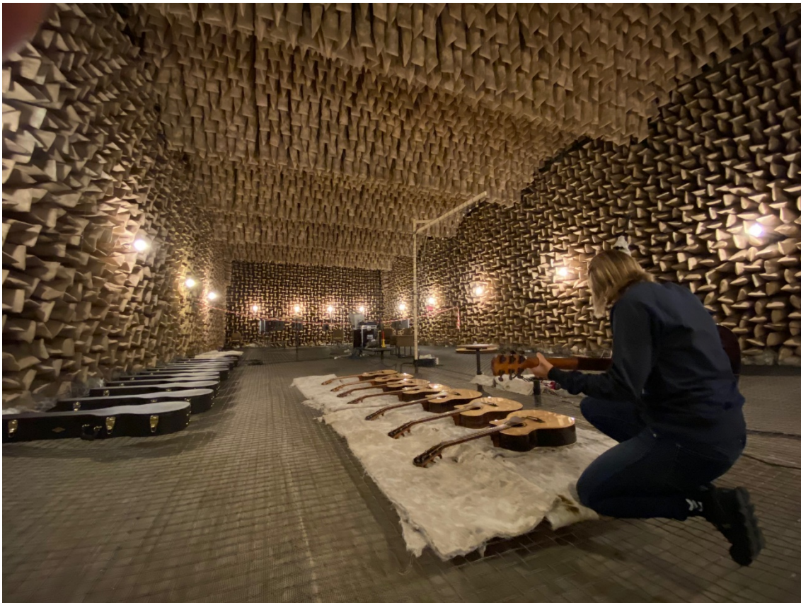
Figure 3 – Final tuning of the guitars in the anechoic chamber.
