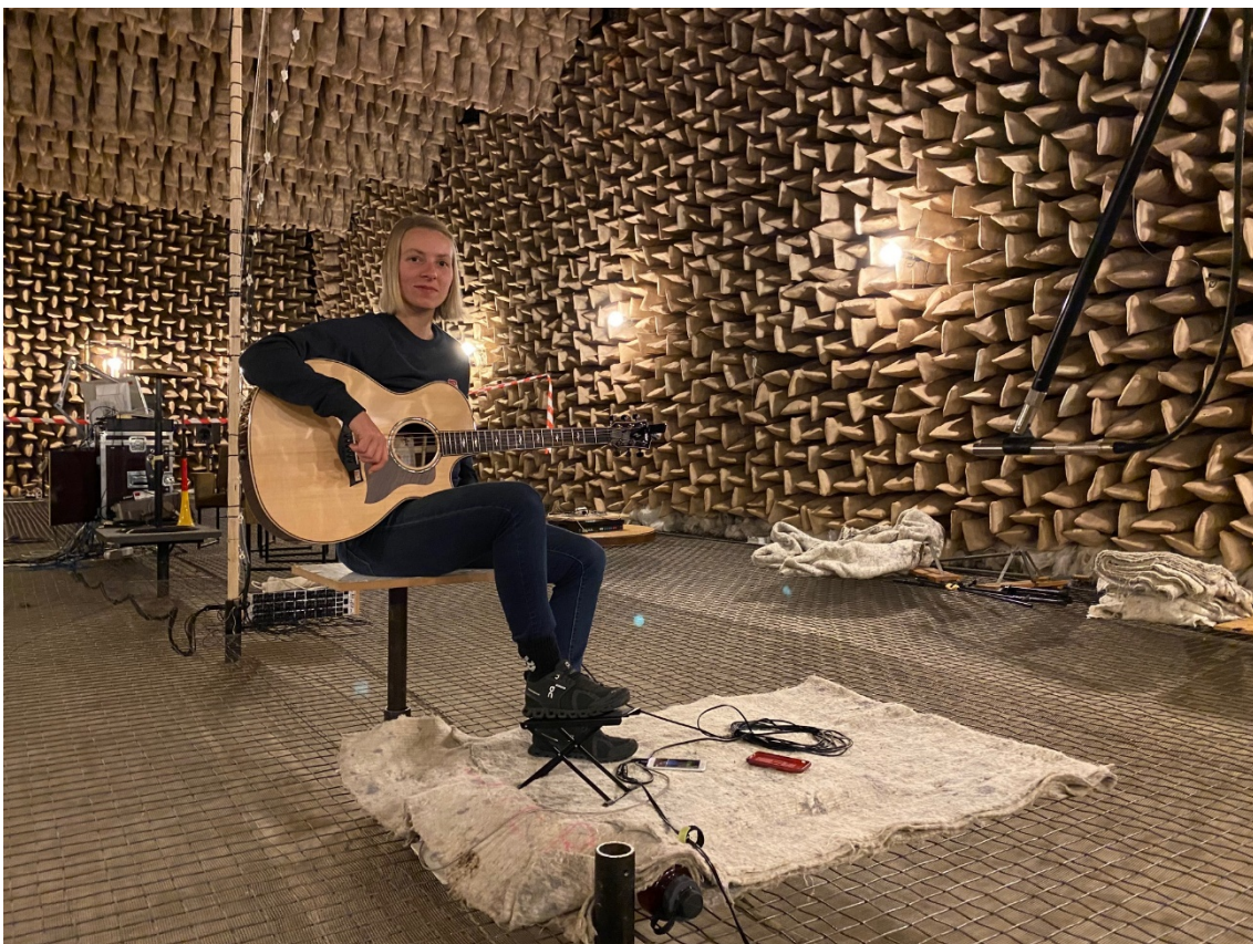
Figure 4 – Recording configuration in the anechoic chamber. The main microphone is positioned 2 m in front of the guitar.
