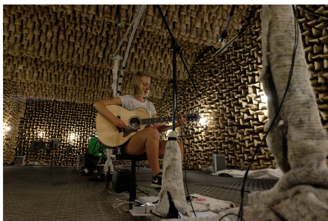
FIG. 4. (Color online) Recording setup in the anechoic chamber. The main microphone position, 2 m in front of the sound hole, can be seen in the top right of the picture. Only this microphone (G.R.A.S. 40HL) was used in the listening tests described in this paper.
